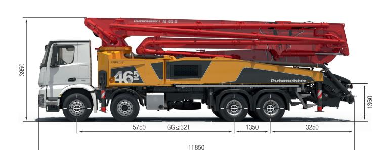
Note: Standard version. Dimensions and weights depend on truck, pump model and equipment. Dimensions in mm, MB-Arocs 4143 as example.
